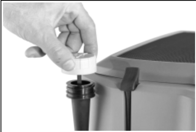
Figure 9-2. Removing Oil Fill Cap/Dipstick.
