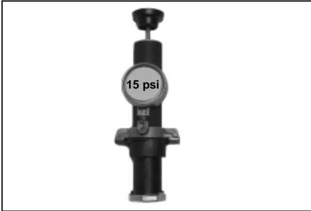
Figure 7-12. Adapter Installed onto the Tester.
