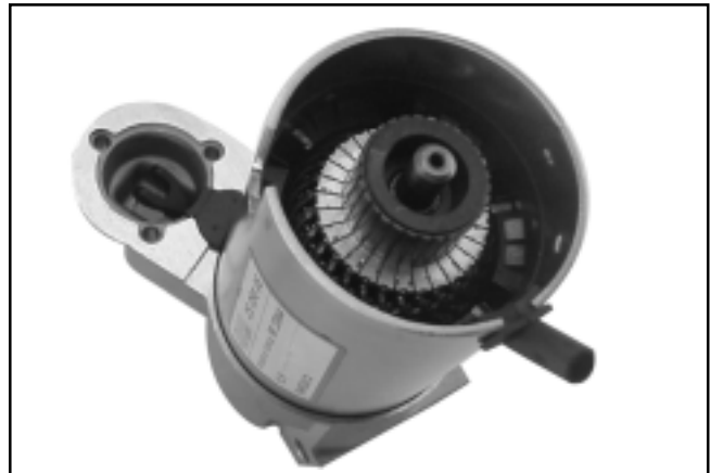
Figure 8-33. Installing Frame and Drain Tube.
