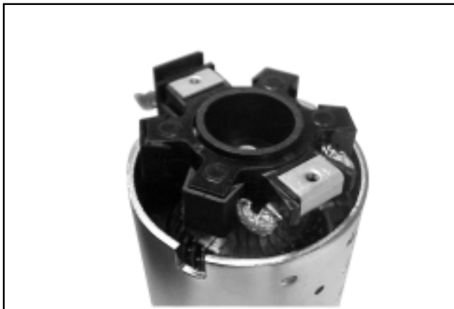
Figure 8-35. Installing Brush Holder Assembly with Supplied Tube.
