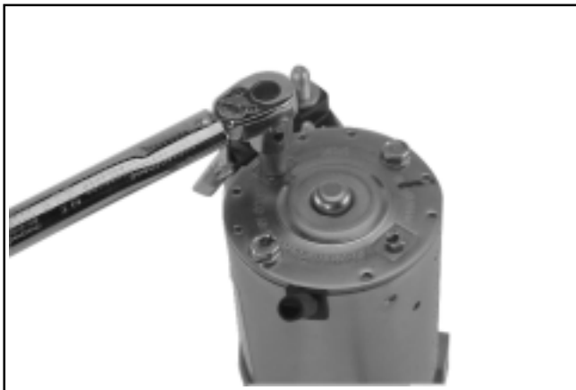
Figure 8-40. Torquing Brush Holder Screws.
