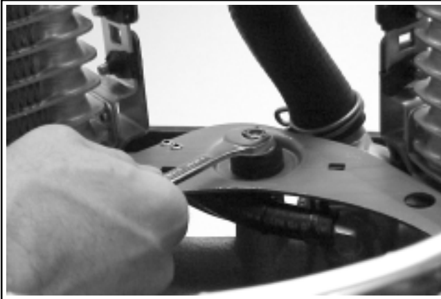
Figure 9-31. Removing Center Mounting Nut.
