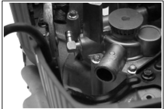
Figure 9-43. Removing By-pass Hose from Water Pump Fitting.
