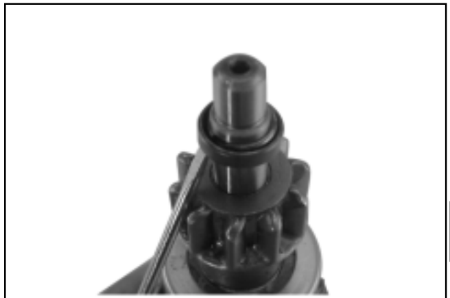
Figure 8-29. Installing Stop Collar and Retainer.
