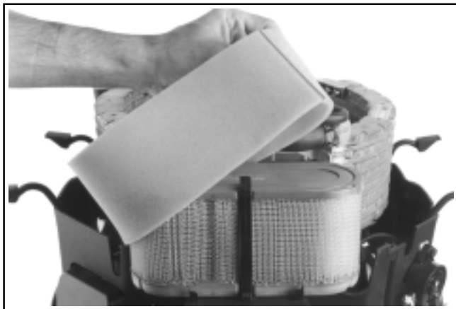
Figure 4-7. Removing Precleaner from Paper Element.
