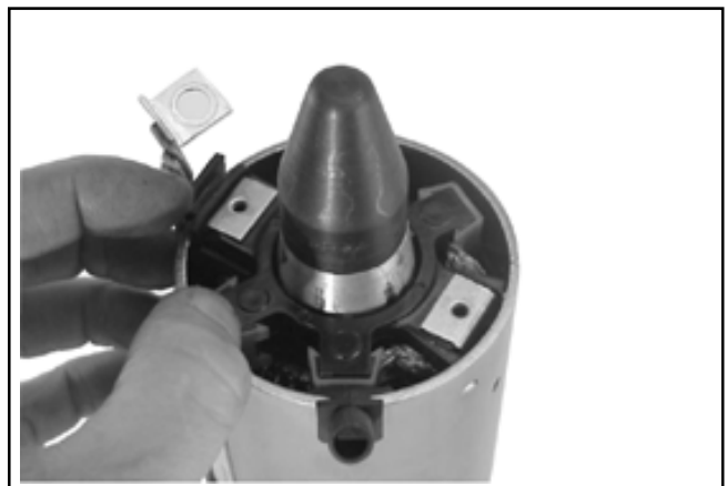
Figure 8-38. Installing Brush Holder Assembly using Tool with Extension.
