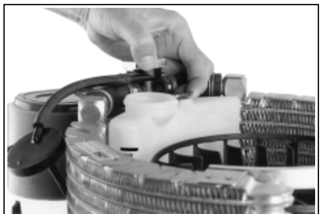
Figure 7-7. Tipping Bracket Away after Removing Reservoir Cap.
