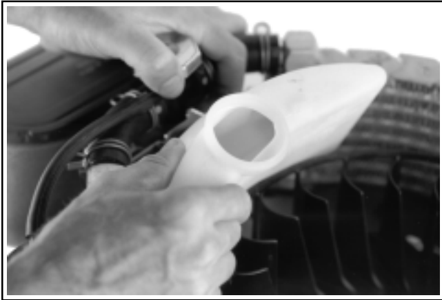
Figure 7-8. Removing Overflow Reservoir.
