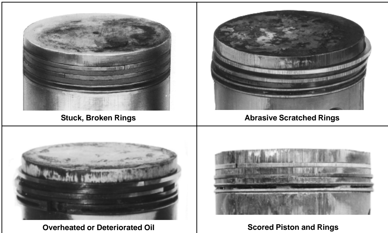
Figure 10-7. Common Types of Piston and Ring Damage.
