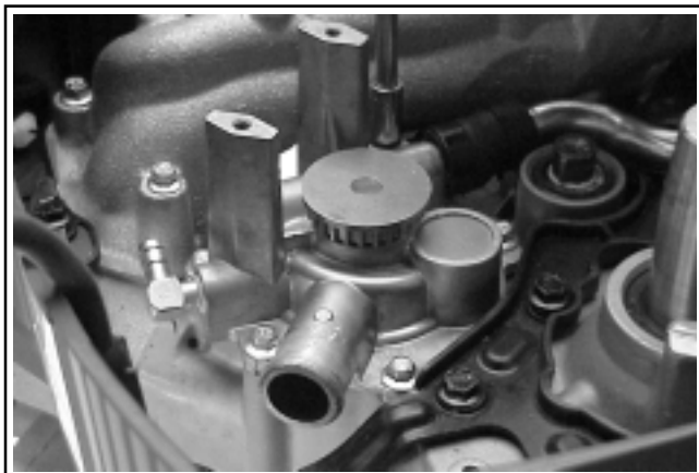
Figure 9-45. Removing the Six Water Pump Screws.
