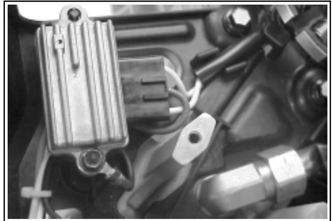
Figure 11-72. Installed Rectifier-Regulator and Wire Routing.
