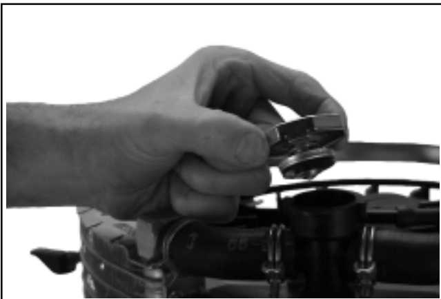
Figure 9-8. Removing Radiator Cap.
