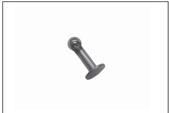
Figure 11-20. Tappet and Ball Bearing Welded Together.
