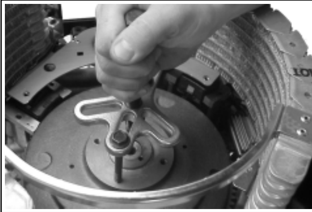
Figure 11-85. Lowering the Flywheel into Position.
