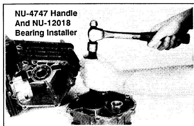
Figure 11-1. Installing Crankshaft Bearings.
