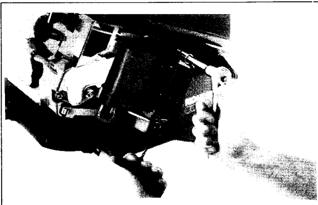
Figure 7-2. Installing Retractable Starter.
