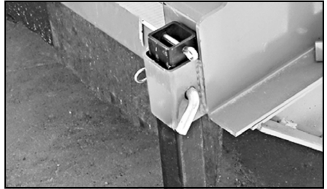
Figure 44. Front Stands Installed
