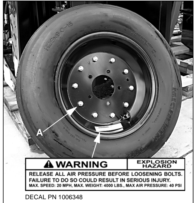
Figure 33. Split Rim Tire Servicing
