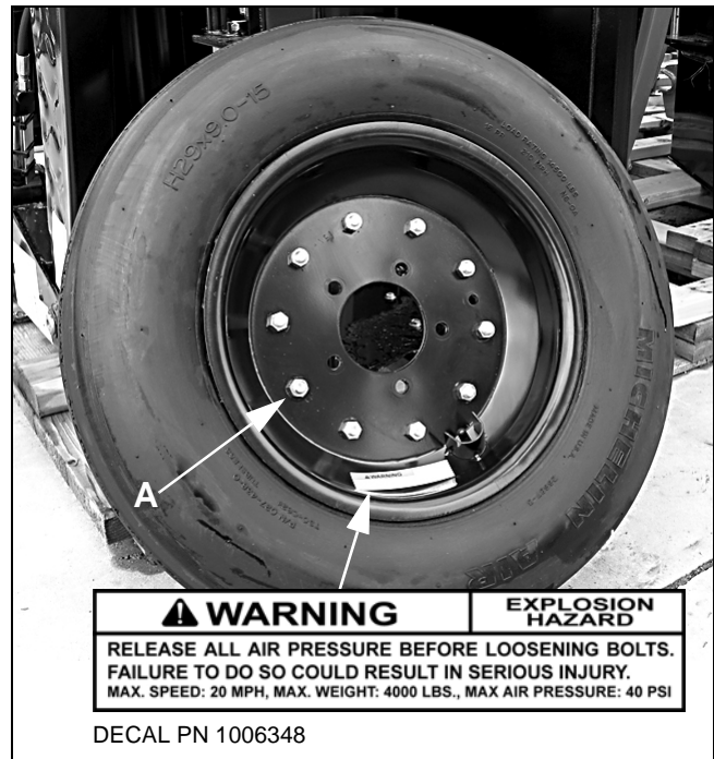
Figure 16. Split Rim Tire Servicing
