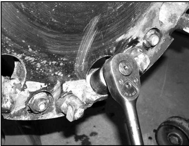
**Figure 6.** Tooth Installed
