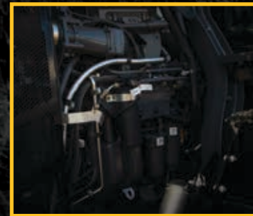
Engine oil can be checked and topped from ground level.
