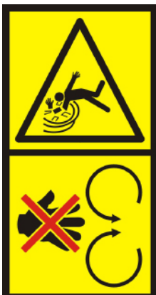
P/N: 379057 WARNING: danger of serious injuries. Do not perform any action on the PTO shaft with the tractor PTO running.
