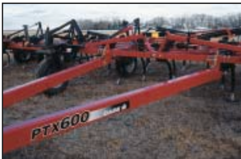
Floating hitch provides improved front to back land following capabilities..
