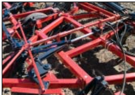
Single cylinder depth control means better reliability, more accuracy and easier maintenance.
