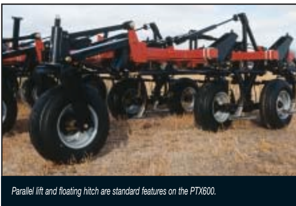
Floating hitch provides improved front to back land following capabilities..
