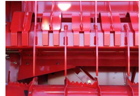
DFCS disengaged for maximum flow through the flywheel.
