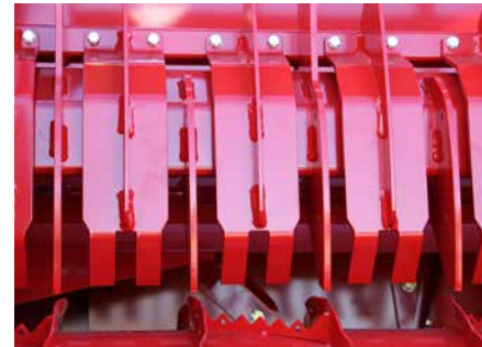
DFCS engaged to reduce the risk of blockages during loading and flywheel start up.
