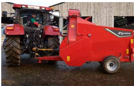
An extended drawbar provides best possible maneuverability during operation. The extended drawbar ensures easier operation, especially when turning with larger tyred tractors.
