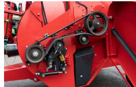
Hydraulic activation of shredder rotor.
