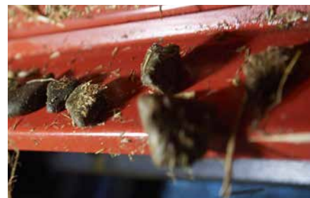
Kverneland 864 features an integrated stone trap positioned at the bottom of the floor conveyor. Foreign objects are separated from the material and easily removed afterwards.
