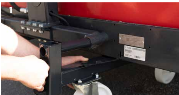
1 Slide the purpose-built transport rollers onto the BX-belt and remove the connection pin.
