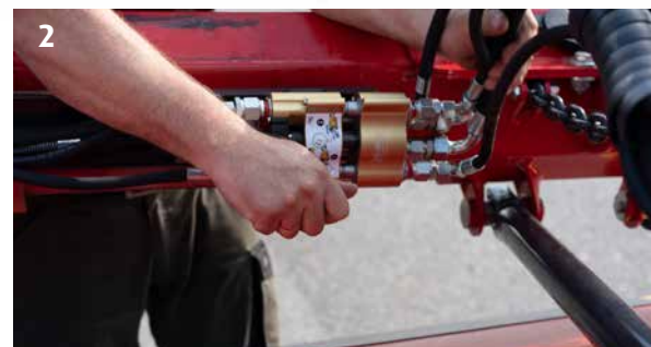
2 Disconnect the power cable and all hydraulic connections to BX belt with one single lever.
