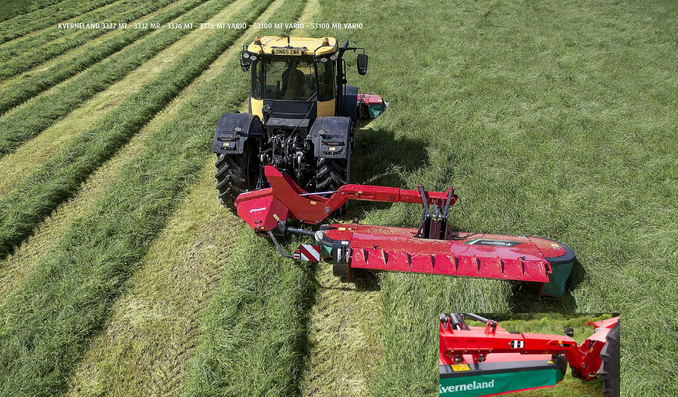
Overlap and effective working width is adjusted hydraulically on Vario models.
