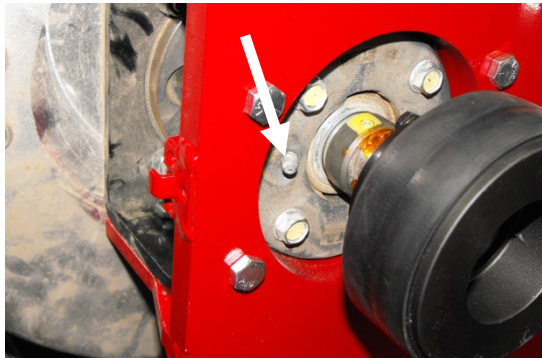
Outside bearing FAN REM HE
