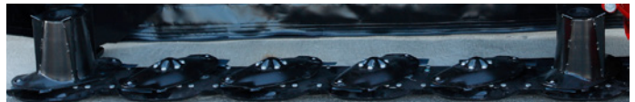
Oval discs allow for superior flow of material over the cutter bar and a better distribution of your hay crop.
