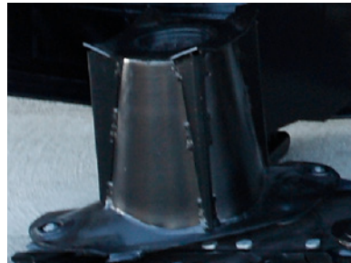
Crop dividers come standard to provide clear distinction between cut and standing hay.
