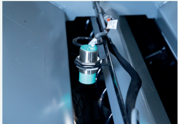
Auxiliary tank leveling system with product level sensors to provide uniform tank product emptying.
