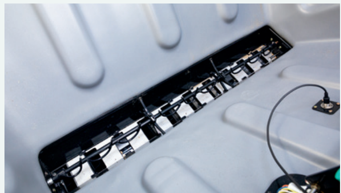
Agitator view inside poly tank. Optional automatic product meter agitation.
