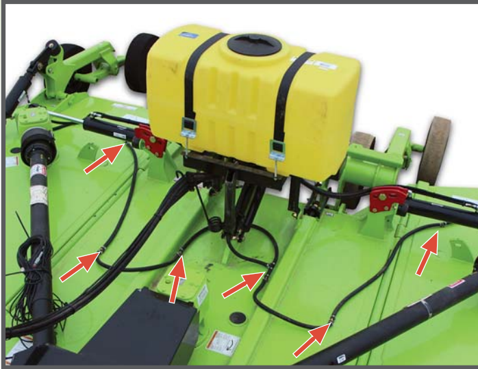
- Arrows Indicate Spray Nozzles -
