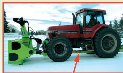
A perfect combination for Schulte's RDX-117 is the FM-300 front mount 3pt hitch frame.
