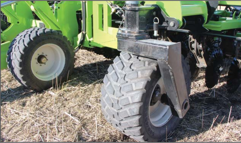
Caster Wheels allow for sharp headland turns and eliminate side skidding. They also help to maintain precise depth control and improve ground following
