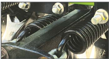
Double heavy duty spring suspension on each disc unit allows for adjustable disc pressure with years of trouble free service
