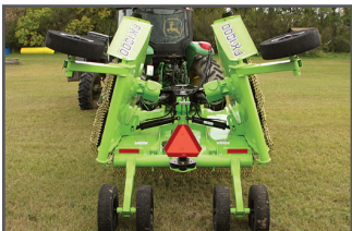
Narrow transport over-centering wing design
