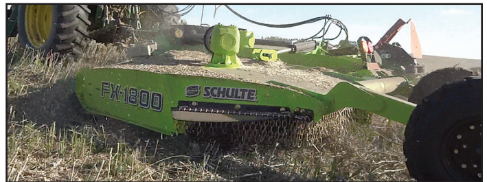
Outboard blade rotation on fixed knife model keeps material from balling up under the deck
