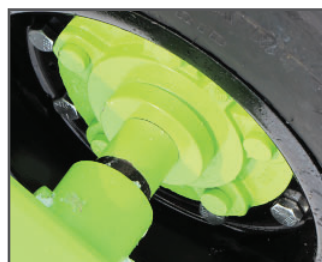
Metal seal guards on 517 hubs
