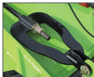
Single levelling rod with floating hitch
