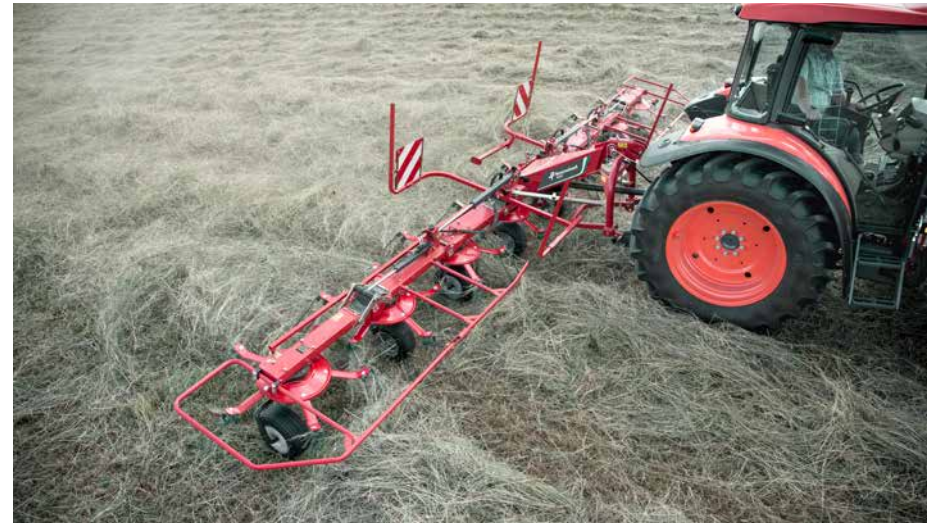
Kverneland 8460-8480 Compact tedders with 6.05 and 8.05m working width - ideal for hay making.
