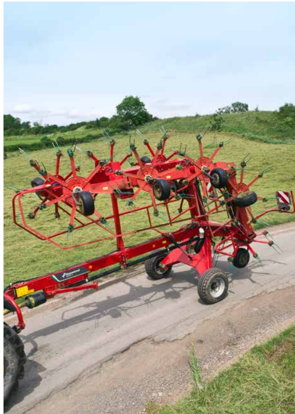
During transport it has a height of only 3.35m and a width below 3.00m.
