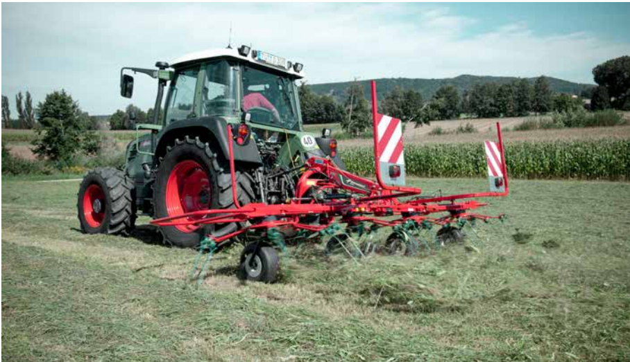
Kverneland 8446-8452-8452 T Compact tedders with low maintenance. Working width of 4.60-5.20m.
