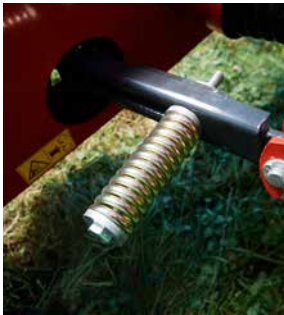
BreakBack device protecting the cutterbar when encountering obstacles.
