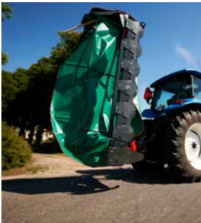
The 2300 series machines are folded hydraulically to a vertical position behind.
