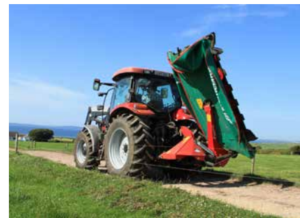
Vertical transport position up to 125°.
