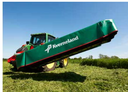
Lifting on headlands via hydraulic cylinder – ample ground clearance.
