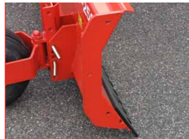
All GT models come standard with the ends prepared for mounting of an end-plate or snow wing.
