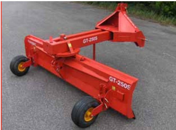
All GT models are prepared for mounting stabilizer wheels, which are easy to adjust individually, without tools, at 25 mm intervals.
