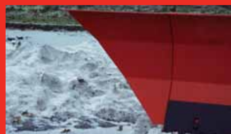
Snow wing that scrapes the edge diagonally so the snow does not fall down behind the scraper.
