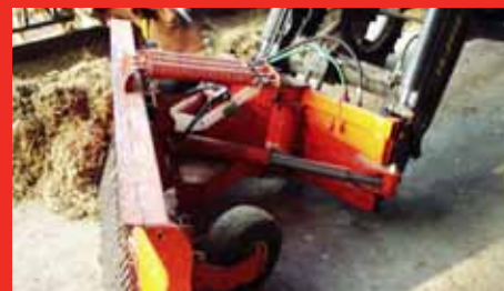
Telescopic cylinder increases the angle of GT-FL scrapers up to 35°.
