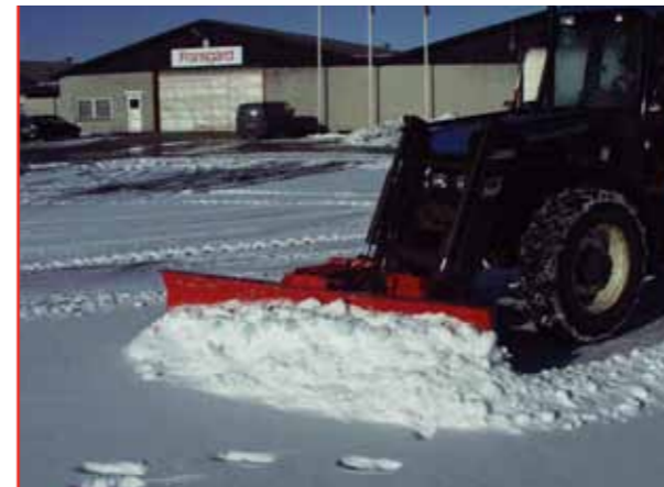
The GT-FL can be mounted on a front hydraulic hitch or a front-end loader. This scraper is perfect for clearing squares, yards or stables. The centermounted scraper creates even pressure on the loader.
