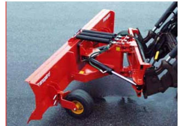
Two robust cylinders are standard and rotate the blade 23° to each side. Overload protection is provided by the three large springs, and the scraper automatically tilts into place after release. All revolving links can be lubricated.
