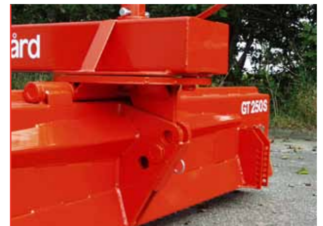
On the GT-250S the scraper's vertical angle can be adjusted offering three blade pitch positions, providing a more aggressive clearing angle. Tool-free manual adjustment.
