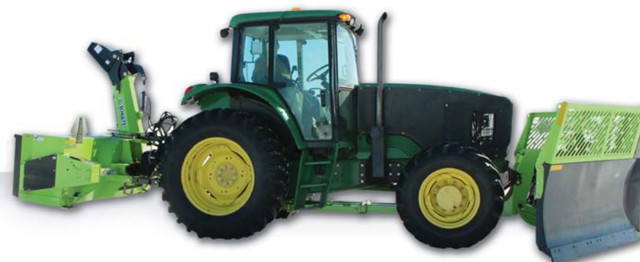
- Front mount frames without drive train allow use of back 3pt hitch -
