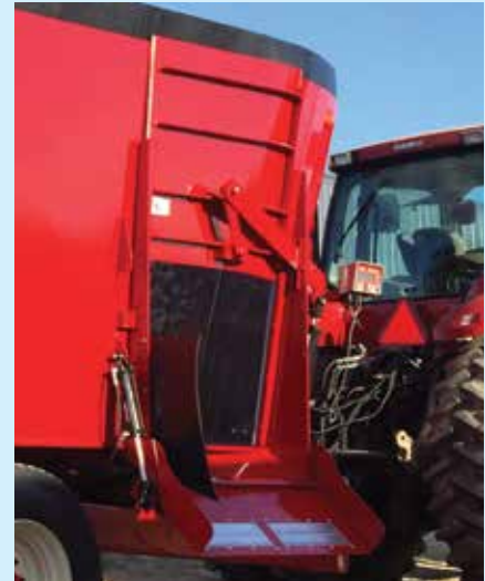
SIDE DOOR - (Left, Right or Both) Pictured with Hydraulic Folding Slide Tray.
