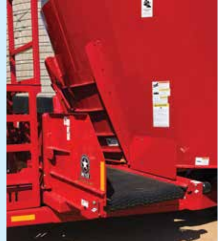
FRONT DOOR - Pictured with Flat Front Belt Conveyor (includes Hydraulic Shift).
