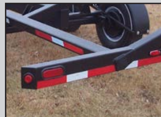
The sealed LED lighting system enables safe towing day and night
