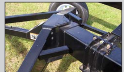
ALL WHEEL STEER HEAD TRANSPORT Heavy duty articulating pivots add strength, durability and provide a short turning radius.
