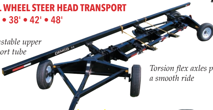
Standard telescoping tongue and EZ Latch 2 5/16" ball coupler and safety chains
