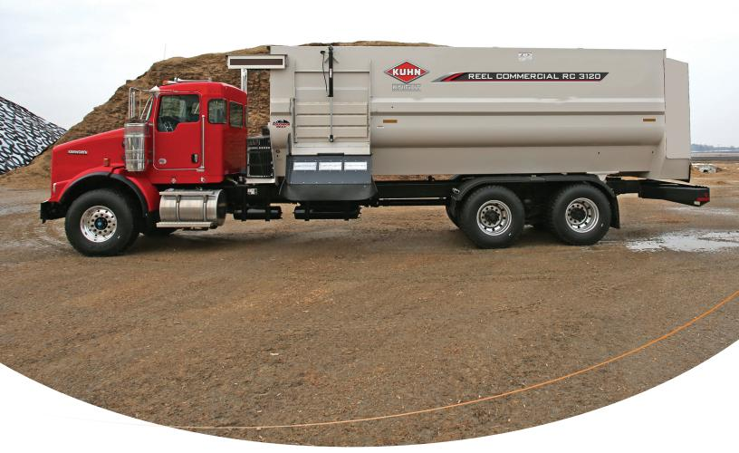
The KUHN Knight RC 3120 is the newest addition to the KUHN Knight reel mixer lineup. Available in truck mount configuration, the RC 3120 boasts a mixing capacity of 1,200 ft³ (34 m³), making it the largest reel mixer offered by KUHN. The large mixing tub features the famous Helix® reel, providing fast, thorough mixing of a wide variety of already processed materials.
