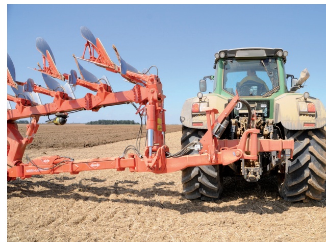
Hydraulic sequencing comes standard meaning fewer valves to operate during headland turns.
