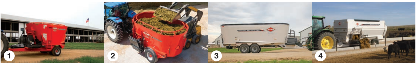
1. Single-auger vertical TMR mixers / 2. Twin-auger vertical TMR mixers / 3. Triple-auger vertical TMR mixers / 4. 4-auger horizontal TMR mixers
