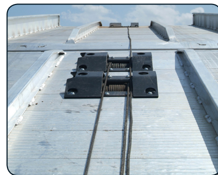
One Winch per Vehicle Upper and Lower Deck
