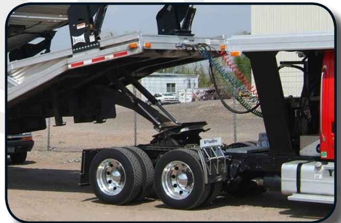
➤ Tilt Cylinder - Major Steel Components Powder Coated
