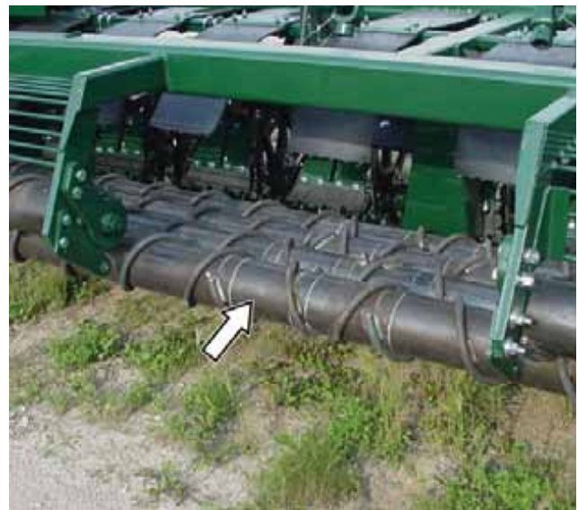
Figure 31. – Header Conveyor Rollers
