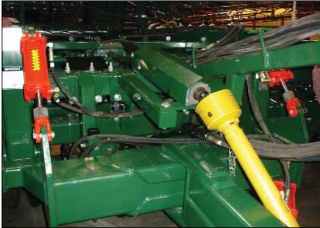
Figure 9. – Hydraulic Connection, Needle Valve Near The Front Left Corner
