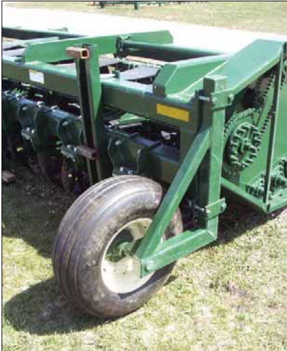
Figure 63. – Front Head Gage Wheels (Standard on 8 row 28/30, 9 row 24/26, and 12 row 22 Heads - Optional on 6 row 22/24, 6 row 28/30, and 8 row 22 Heads)
