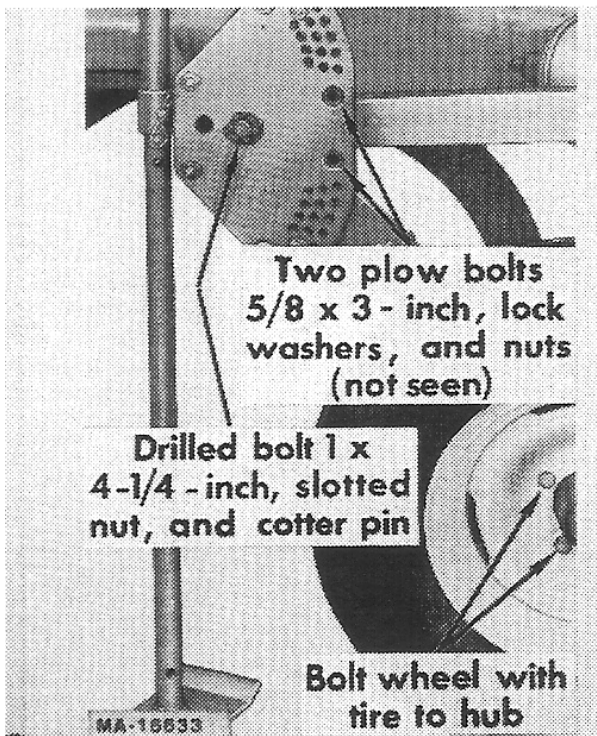
Figure 33 - Three And Four Furrow Rigid And Spring Trip Plows
