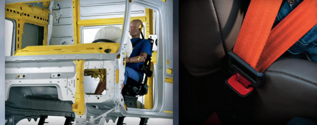
The VNM 200, 430 and 630 come standard with the industry's leading collision protection technology. In the event of an accident, the High Strength Steel Cab and three-point safety harness protect the driver while the airbag deploys. The engine and transmission are designed to drop down and away from the driver as the steering column automatically collapses.
