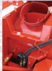
DRUM ROTATION MECHANISM WITH HYDRAULIC MOTOR ON ALL MODELS
