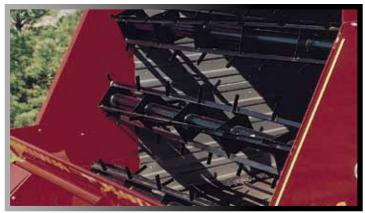
H&S uses three – 18" 4 bar H.D. spiral type beaters – not augers. Aggressive in handling tough material, they are even feeding. All three beaters are mounted in the head, not auxiliary panels in the box. Beater shafts are  $1\frac{1}{4}$ " equipped with greasable bearings.
