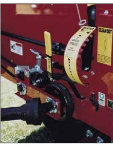
A separate clutch allows you to start and clear the beaters before you start the main apron conveyors. The HD clutch can be used to engage just the cross conveyor, the cross conveyor and beaters, or the cross conveyor, beaters and main floor apron in any speed.
