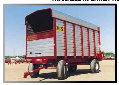
H&S engineered this box for bulk hauling and unloading in bunk or pit storage facilities. Available in trailer or truck mounts.
