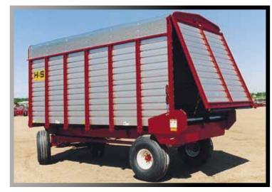
The heavy duty tailgate is constructed to stand up to the pounding of heavy loads. High pivot points assure crop clearance while unloading.
