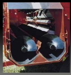
The twin auger utilizes two – 10" high speed cross augers equipped with hold-downs and wipers. The auger housings are poly-lined to reduce build-up.
