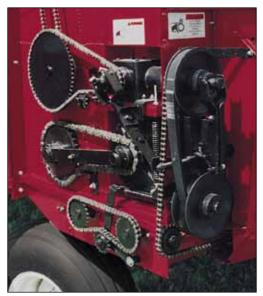
A simple trouble-free variable speed drive lets you match just the right unload speed to the crop type, load condition and blower capacity.
