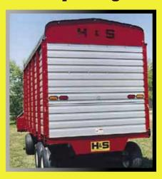
Transport lights are standard on all H&S boxes. Above is the light configuration on front unload boxes. Below is the configuration for rear unload boxes.
