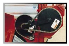
The H&S power box can be ordered with either a P.T.O. drive or a hydraulic drive. Unload time is dependent on tractor R.P.M., hydraulic pressure, and G.P.M.
